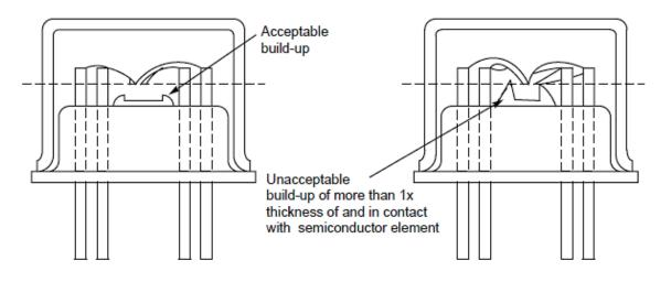
DETAIL A 2x semiconductor element height maximum
