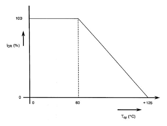
Rated Contact Current versus Temperature
