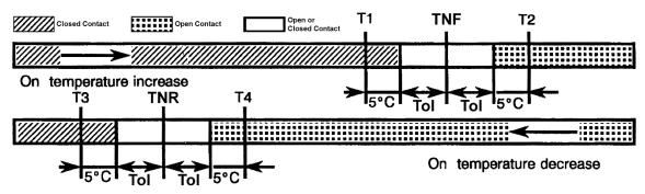
For a Switch with Closing Contact:
