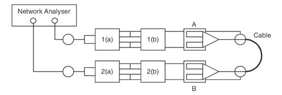
1(a) and 2(a) : Symmetrical Transformers (1 x  $50\Omega$  to 2 x  $50\Omega$ )
