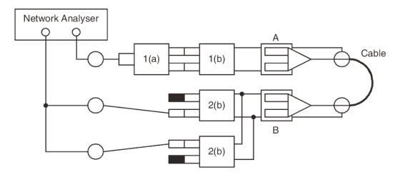
1(a) and 2(a) : Symmetrical Transformers (1 x  $50\Omega$  to 2 x  $50\Omega$ )
