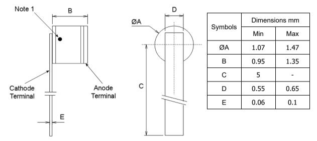
Terminal identification: The body shall be marked at a suitable location near the cathode terminal with a black dot.
