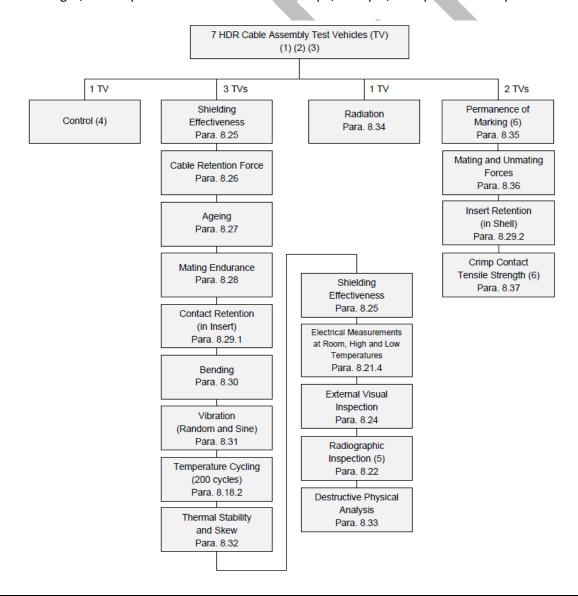
Based on the qualification philosophy and on the test sequences required by ESCC no. 3409, the test vehicles were designed to be representative of the use.
