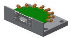
For TV no. 3 (parallel gap connector mated with blanking plate), the 3 samples are tested during the same vibration run. The 3 samples are fixed on the same angle bracket, positioned on the vibration plate during a vibration run of a TV no.1 sample.
