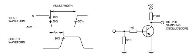
4.  $t_{off}$  shall be measured using the following test circuit. The input waveform shall be supplied by a pulse generator with the following characteristics:  $Z_{OUT} = 50\Omega$ ,  $t_f \le 2$ ns, Pulse Width = 10 to 100 $\mu$ s, Duty Cycle  $\le 2$ %. The output waveform shall be monitored on an oscilloscope with the following characteristics:  $Z_{IN} \ge 100$ k $\Omega$ , input capacitance  $\le 12$ pF,  $t_r \le 5$ ns.
