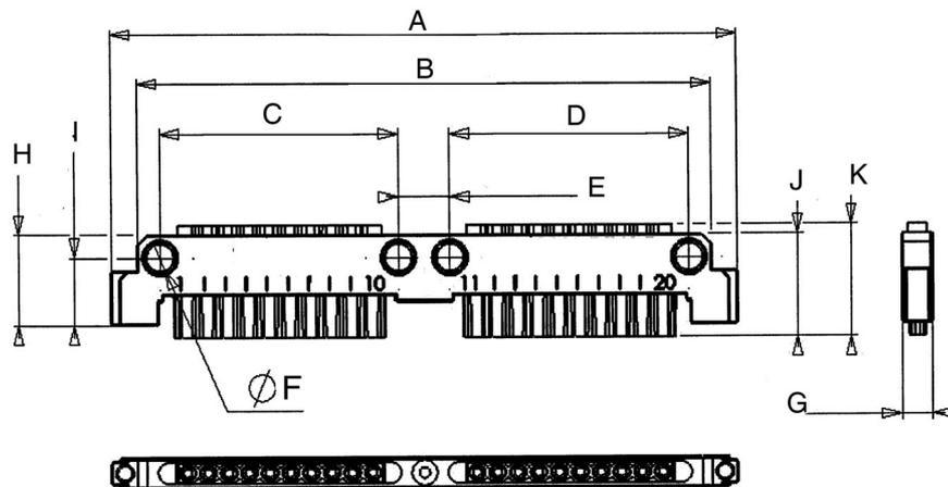
CONTACT ARRANGEMENT - 20 female size AWG 20 contacts
