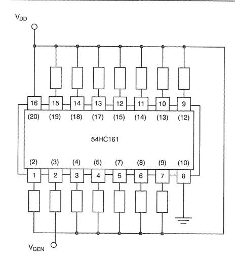
**NOTES** 1. Pin numbers in parenthesis are for the chip carrier package.
