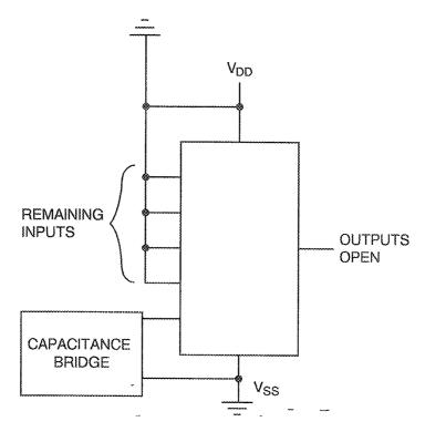
**NOTES** 1. Each input to be tested separately. 2. f = 100KHz to 1MHz.
