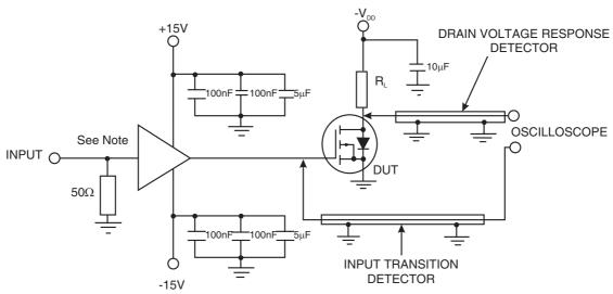
$\begin{tabular}{ll} {\bf NOTE:} \\ {\bf The amplifier shall be a suitable voltage follower/buffer amplifier.} \\ {\bf VOLTAGE \ WAVEFORMS} \\ \end{tabular}$
