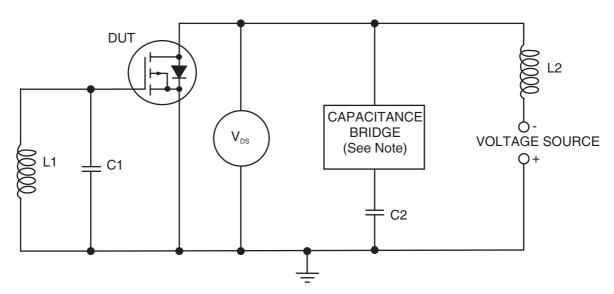
**NOTE:** The capacitance bridge shall have low DC resistance between its output terminals and should be capable of carrying the test current without affecting the desired accuracy of measurement.
