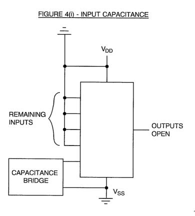
**NOTES** 1. Each input to be tested separately. 2. f = 100KHz to 1MHz.
