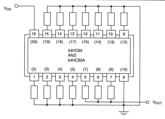
**NOTES** 1. Pin numbers in parenthesis are for the chip carrier package.
