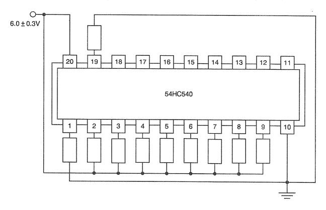
NOTES 1. Input Protection Resistor = 680Ω min. to 47kΩ max.
