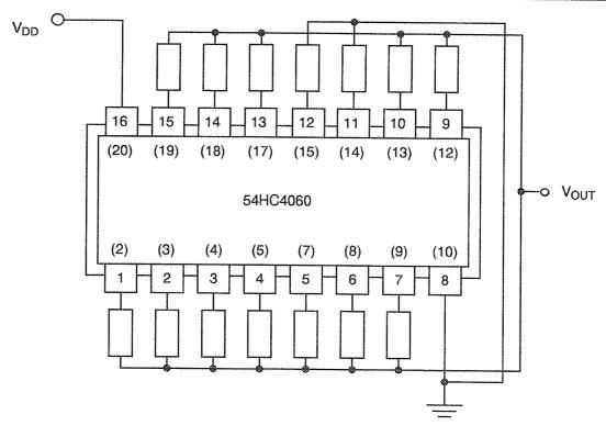
**NOTES** 1. Pin numbers in parenthesis are for the chip carrier package.
