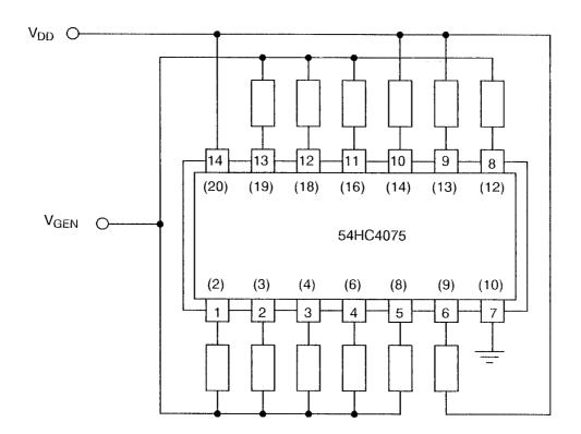
$\underline{\textbf{NOTES}}~~1.~$  Pin numbers in parenthesis are for the chip carrier package.
