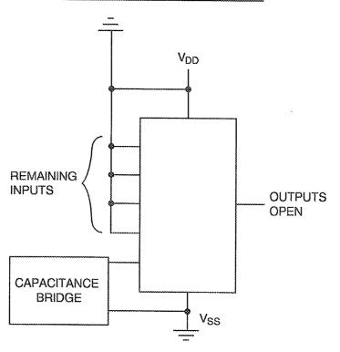
**<u>NOTES</u>** 1. Each input to be tested separately. 2. f = 100KHz to 1MHz.
