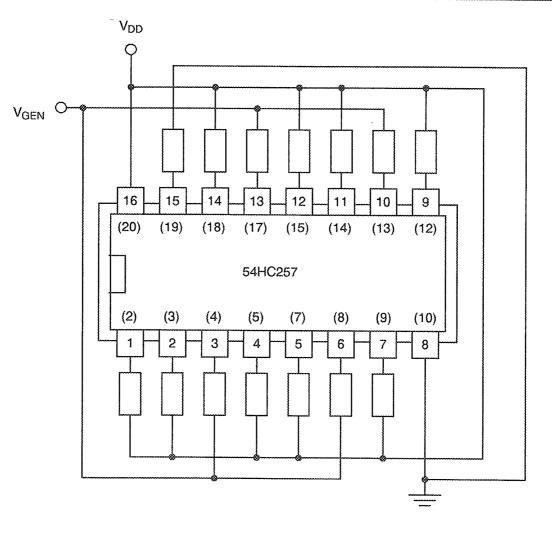
NOTES 1. Pin numbers in parenthesis are for the chip carrier package.
