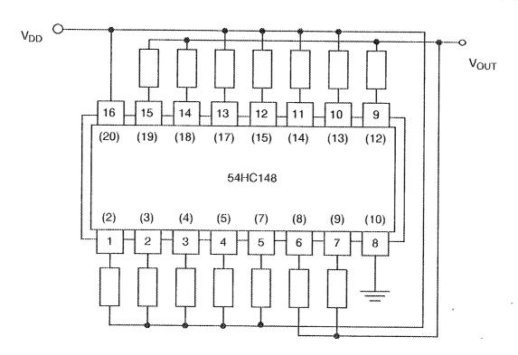
**NOTES** 1. Pin numbers in parenthesis are for the chip carrier package.
