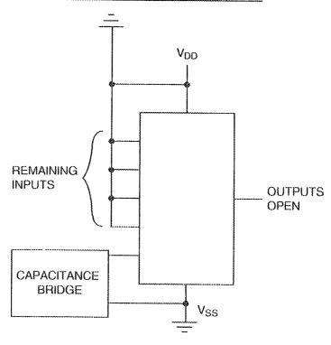
NOTES 1. Each input to be tested separately. 2. f = 100 KHz to 1 MHz.
