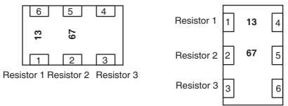
For arrays with 4 to 8 resistors, the marking shall be located adjacent to the first 4 resistors of the array. The first resistor,  $R_1$ , of the array is on the left hand end of the array whilst reading the marking, as follows:
