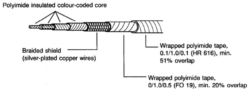
**FIGURE 2(c) - SHIELDED AND JACKETED CABLES**
