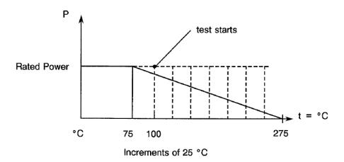
For each step, the temperature shall be allowed to stabilise and the resistors shall remain under these conditions for 1.5 hours. Case temperatures shall be monitored by means of thermocouples and be recorded after one hour of stabilised conditions. Following the 1.5 hour time lapse, the resistors shall be taken out of the chamber and allowed to cool at room temperature for a period of two hours. The resistance shall then be measured and the resistors be examined visually.
