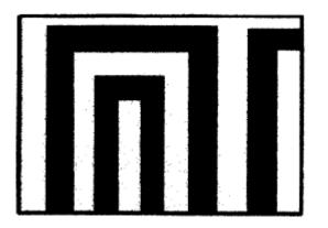
**<u>GOOD</u>** No visible point of delamination.
