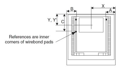
X and Y define the centre of the 576 x 780 array of active elements. X and Y' define the centre of the minimum imaging 514 x 740 pixels. A, B and C are measured from the optical references.
