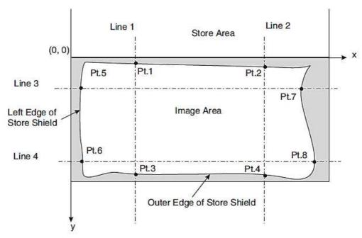
Lines 1, 2, 3 and 4 are at 1/4 and 3/4 across the image area in each direction. Points 1, 2, 3,..., 8, with coordinates (x1, y1), (x2, y2), etc., are the locations of the 50% threshold pixels (see above). The coordinates of these points are used to calculate, in pixels, the average Left, Right, Outer and Store Edge positions and Shield Rotation as follows:
