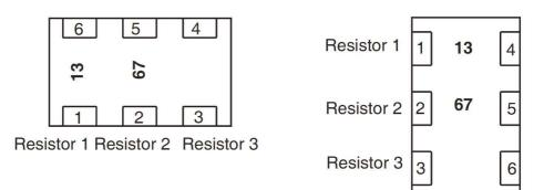
For arrays with 4 to 8 resistors, the marking shall be located adjacent to the first 4 resistors of the array. The first resistor,  $R_1$ , of the array is on the left hand end of the array whilst reading the marking, as follows:
