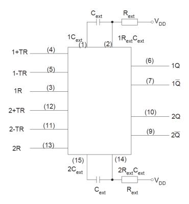
$\label{eq:rescaled} \begin{array}{ll} \underline{\text{NOTES:}} \\ 1. \quad C_{\text{ext}} \leq 100 \mu F; \ R_{\text{ext}} \geq 5 k \Omega \end{array}$
