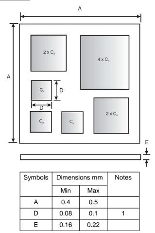
NOTES: 1. Dim Dimension of the smallest bond pad area, specified for bonding purposes.
