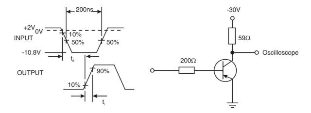
4.  $t_s$  and  $t_f$  shall be measured using the following test circuit. The input waveform shall be supplied by a pulse generator with the following characteristics:  $Z_{OUT} = 50\Omega$ ,  $10\mu s \le Pulse$  Width  $\le 500\mu s$ ,  $t_r = t_f \le 2ns$ , Duty Cycle = 2%. The output waveform shall be monitored on an oscilloscope with the following characteristics:  $Z_{IN} \ge 100k\Omega$ ,  $t_r \le 200ps$ ,  $C_{in} \le 12pF$ .
