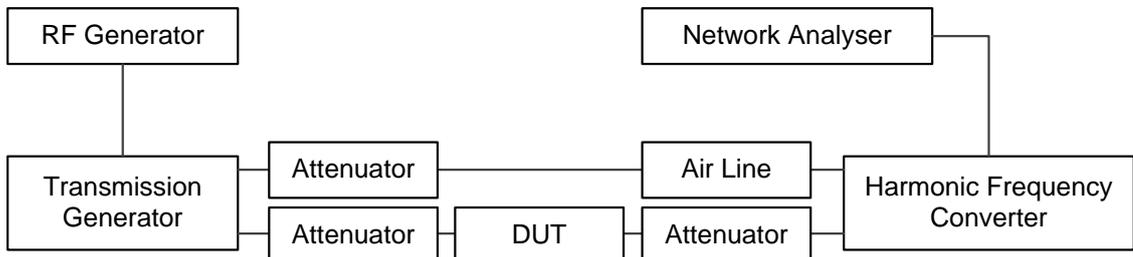
**FIGURE III - SWEEP FREQUENCY VSWR TEST SET-UP**
