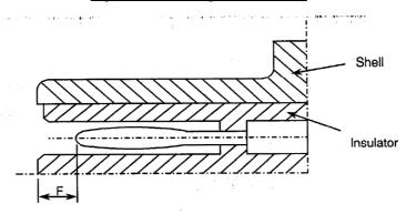
Figure 2.2.3 – Receptacle Female Contact
