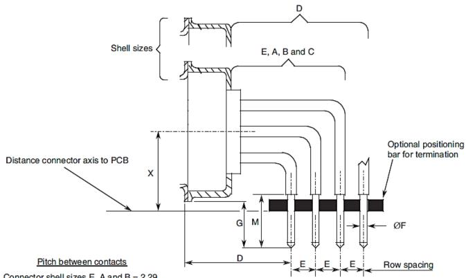
Connector shell sizes E, A and B = 2.29. Connector shell sizes C and D = 2.41.
