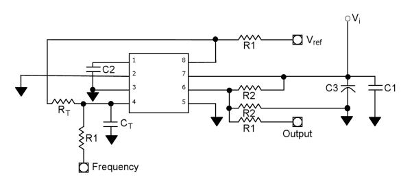
$R_T = 10k\Omega \qquad \qquad C_T = 470pF$   $R1 = 1k\Omega \qquad \qquad C1 = 100nF$   $R2 = 100k\Omega \qquad \qquad C2 = 1\mu F$   $C3 = 470\mu F$
