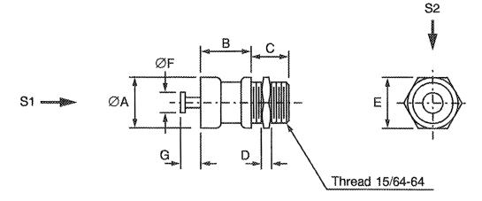
S1, S2 – Vibration and Shock axes
