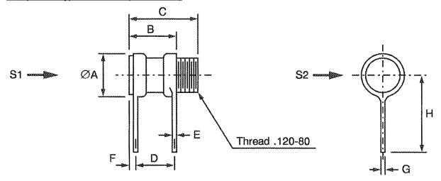
S1, S2 - Vibration and Shock axes
