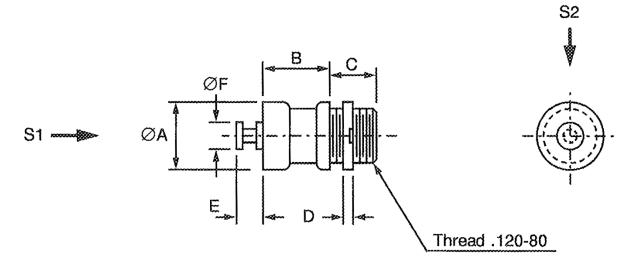
S1, S2 - Vibration and Shock axes
