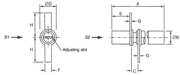
S1, S2 - Vibration and Shock axes
