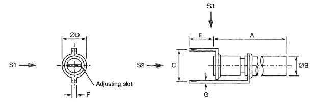
S1, S2, S3 - Vibration and Shock axes
