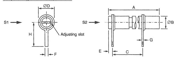
S1, S2 - Vibration and Shock axes
