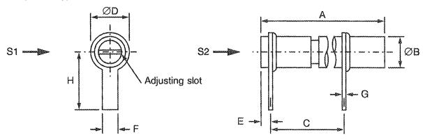
S1, S2 - Vibration and Shock axes
