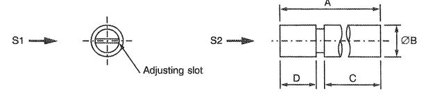
S1, S2 - Vibration and Shock axes
