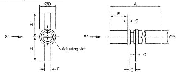
S1, S2 - Vibration and Shock axes
