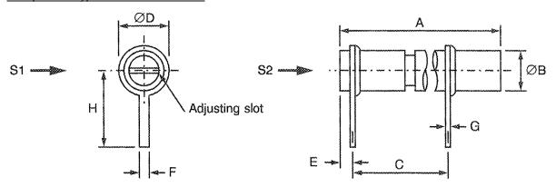
S1, S2 - Vibration and Shock axes
