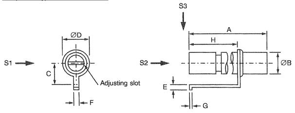
S1, S2, S3 - Vibration and Shock axes
