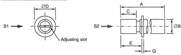
S1, S2 - Vibration and Shock axes
