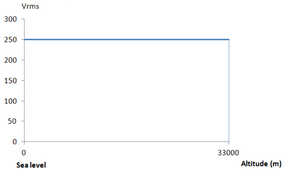
FIGURE 1(a) – WORKING VOLTAGE VERSUS ALTITUDE
