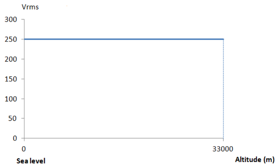
FIGURE 1(a) – WORKING VOLTAGE VERSUS ALTITUDE
