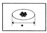
ACCEPTABLE Wire is slightly flattened. Rule:  $\emptyset \le 1.4 \times \text{Nominal diameter}$ .
