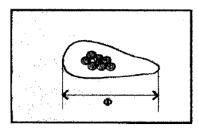
$\frac{\textbf{REJECTED}}{\text{Wire is flattened.}}$ Rule:  $\emptyset > 1.4 \times \text{Nominal diameter.}$
