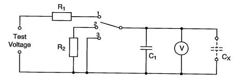
The resistance of the voltmeter shall be not less than 10 000 $\Omega$ /V.
