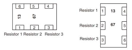
For arrays with 4 to 8 resistors, the marking shall be located adjacent to the first 4 resistors of the array. The first resistor,  $R_1$ , of the array is on the left hand end of the array whilst reading the marking, as follows:
