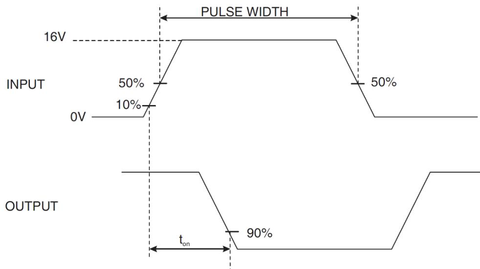
4.  $t_{off}$  shall be measured using the following test circuit. The input waveform shall be supplied by a pulse generator with the following characteristics:  $Z_{out} = 50\Omega$ ,  $t_r \leq 2\text{ns}$ , Pulse Width =  $10\mu\text{s}$ , Duty Cycle  $\leq 2\%$ . The output waveform shall be monitored on an oscilloscope with the following characteristics:  $Z_{in} \geq 100\text{k}\Omega$ , input capacitance  $\leq 12\text{pF}$ ,  $t_r \leq 5\text{ns}$ .
