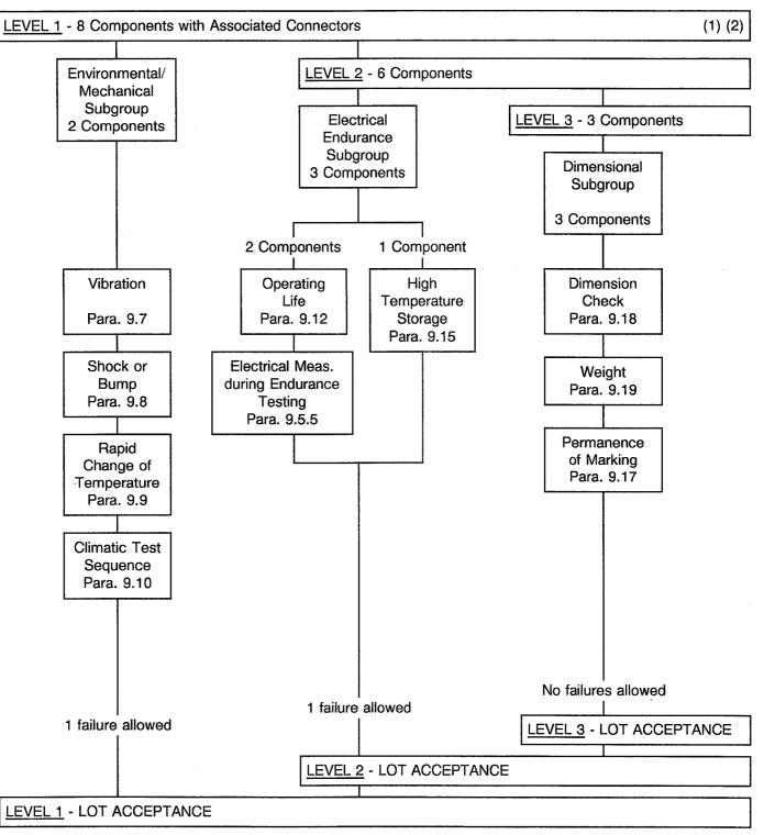
Total allowable number of failed components: 1 (which shall not be in the Dimensional Subgroup).
