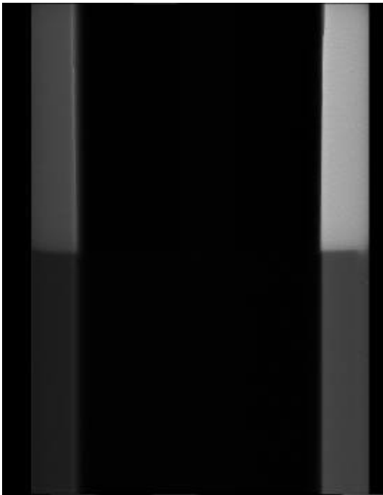
Figure 5.5.4-4 Full frame image for CCD #3 showing increased dark current for the storage region (top of image), 8°C, 500 ms integration time.
