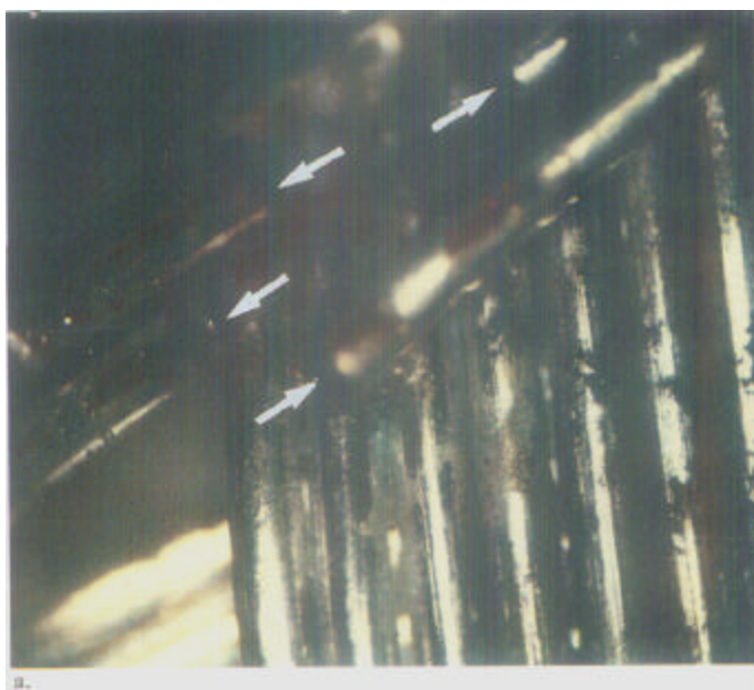
Figure 2. Colour photomicrographs of typical 'red-plague' corrosion areas on braiding, as circled in Figure 1.
