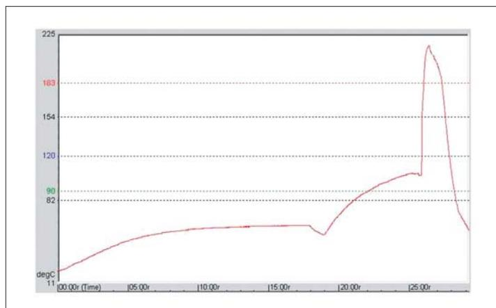
Figure 14. Typical temperature profile achieved for vapour-phase soldering
