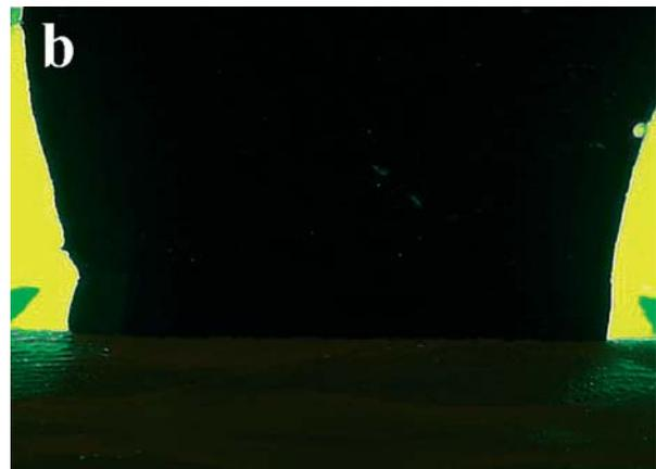
*Figure 17. Cross-sections of corner solder joints showing the laminate beneath the solder pads on boards soldered using low (a) and high (b) peak temperature examined with UV light*
