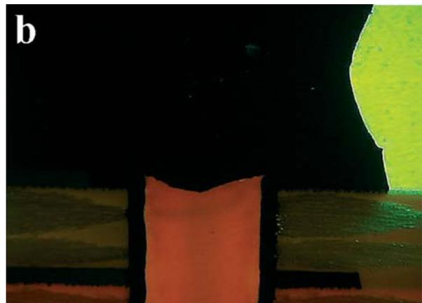
Figure 21. Cross-sections of corner solder joints showing the laminate beneath the solder pads on boards with via-in-pad design from Manufacturers X (a) and Y (b) examined with UV light
