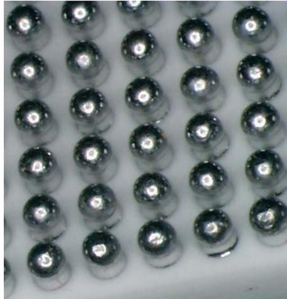
Figure 5. Photograph showing some of the balls on a ceramic BGA
