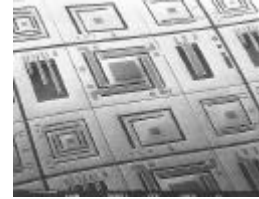
SEM photograph of the chip with different bimorphous actuators. The HRXRD measurements were executed on the middle plate of the fourfold symmetrical structure in the middle of the photograph.
