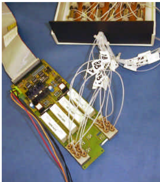
Figure 4: The "MUSE system". At the development of the system, COTS (commercially available) electronics has been applied. The flight hardware will be up to 50% smaller.
