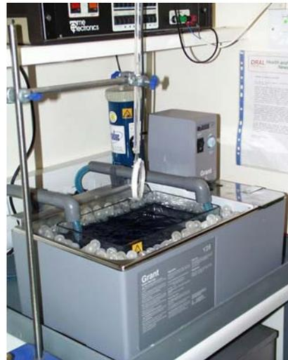
**Figure 9 - Electroplating bath and motorised arm assembly.**
