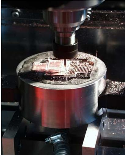
**Figure 11 - Machining of collimators.**
