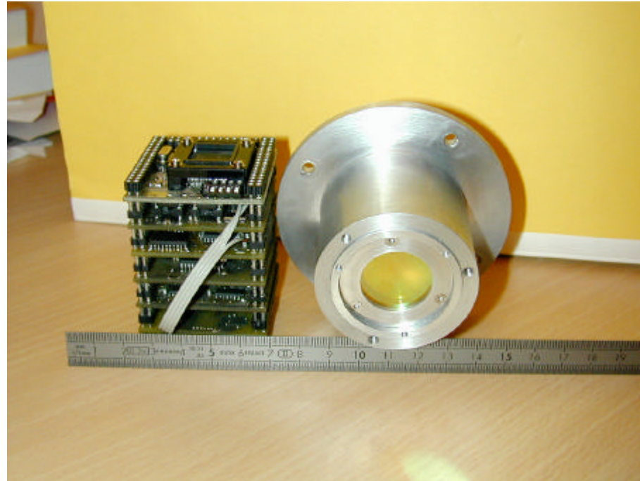
MIREs : MicroEarth Sensor developed by the LAAS-CNRS (CNES project) (Volume:electronics 80 cm 3 , optics 24 cm 3 )
