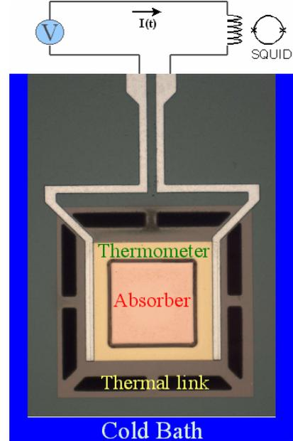
Figure 1 Annotated micrograph of a single pixel X-ray microcalorimeter, used for explanation of the operation principle (see text).
